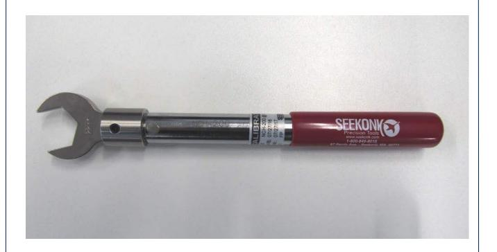
Pre-set at factory to desired value within a  $\pm$ -4% tolerance. When preset torque value is achieved, a distinct click is felt and heard, followed by a sudden release into several degrees of free movement. Ideal for applications in which one torque value is used extensively. Compact design makes these tools invaluable in hard to reach locations. Tools automatically reset when torquing-force is removed.
