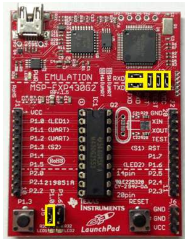
Figure 3. Proper Jumper Configuration on the LaunchPad
