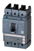
circuit breaker 3VA5 UL frame 250 breaking capacity class H 65kA @ 480V 2-pole, line protection TM210, FTFM, In=100A overload protection Ir=100A fixed short-circuit protection li=10 x In without connection
