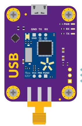
Connect Flow breakout board to the carrier board.
