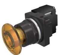
30mm BlackMax, Epoxy Coated Corrosion Resistant Metal Operator, Round Illuminated Twist-to-Release Full Voltage, 24V AC/DC LED Lamp Mushroom Head Cap Small 1.79" (45 mm) Plastic Cap, Amber 2 Position Maintained, Twist-to-Release UL Listed, CSA Certified NEMA 1,3,3R,4,4X,12,13 & Automotive Standards
