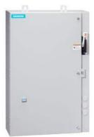
Non-reversing motor starter Size 2 1/2 Three phase full voltage Solid-state overload relay OLRelay amp range 25-100A 110-120/220-240VAC 60HZ coil Combination type 100A circuit breaker Enclosure NEMA type 4/12 Water/dust tight for outdoors Standard width enclosure
