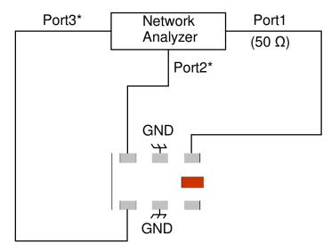
\*Impedance for ports 2 and 3=1/2(Balanced impedance)
