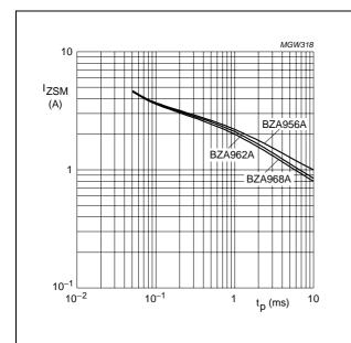
Fig.2 Maximum non-repetitive peak reverse current as a function of pulse time.
