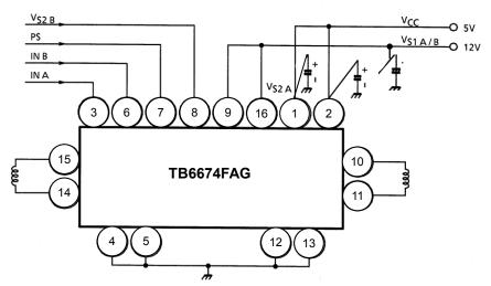
Note 1: Connect the  $V_{\mbox{S2A}}$  terminal to the lower supply voltage (5 V).
