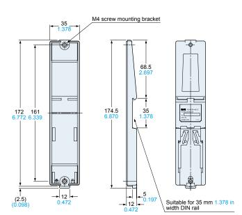
Two M4 (length 12 mm 0.472 in) screws with washers are attached.
