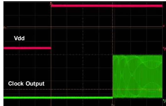
Figure 17. Startup Waveform vs. Vdd
