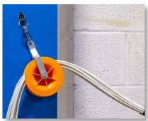
The CP-475 is a set of two cable pulleys designed to help install electrical, COAX, network, and other various low voltage cables. With their swivel snap hooks, deep grooves, and anti-friction bearings, these pulleys keeps cables aligned with the direction of the pull, preventing snags and kinks.
