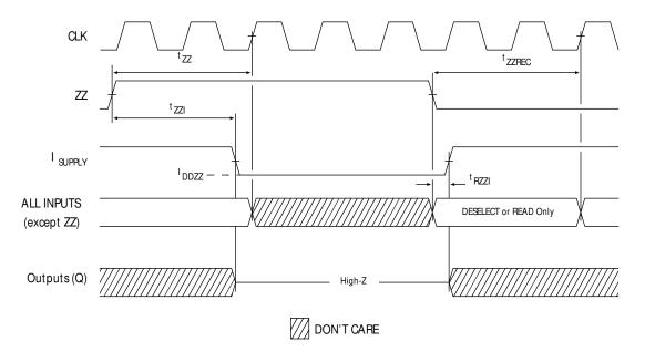
25. Device must be deselected when entering ZZ mode. See truth table for all possible signal conditions to deselect the device. 26. DQs are in high-Z when exiting ZZ sleep mode.
