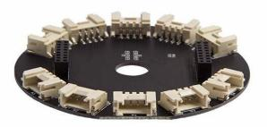
Up to 10 Grove Ports: I2C, UART, Digital I/O, Analog I/O Stackable with ReSpeaker Core and ReSpeaker Mic Array Highly Extendible with Two 2 x 8 headers
