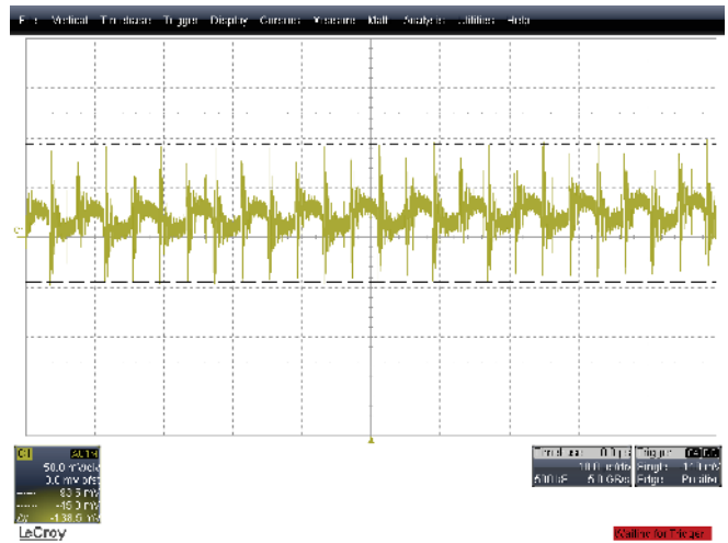
Figure 25. UCC29950EVM-631 Output Noise (230- V_{AC} , 50-Hz input, full load)
