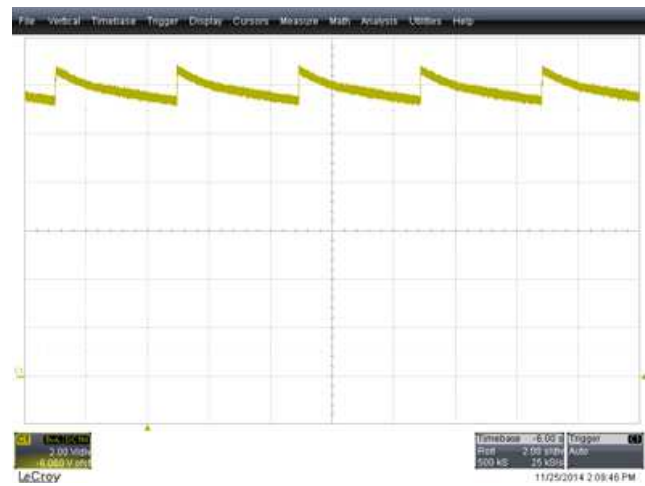
Figure 27. V_{OUT} , No Load, Self Bias, Burst Interval is 4-s intervals, \Delta V_{OUT} = 1.5 V
