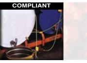
1) In areas where we transfer flammable liquids, are we missing the means to effectively ground and bond the containers?
