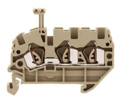
Feed-through terminal, Tension-spring connection, Mounting type: Mounting rail TS 35/7.5, Rated cross-section: 2.5 mm², Width: 5.1 mm, Colour: Beige
