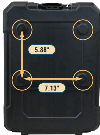
MOUNTING BOLT PATTERN
