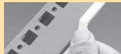
Picture 1 - Proper way to remove CHO-MASK mask
