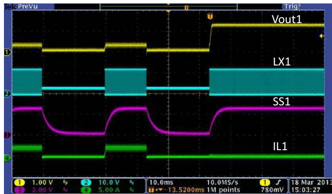
Figure 34. Hiccup Recover, Buck1=1.2V
