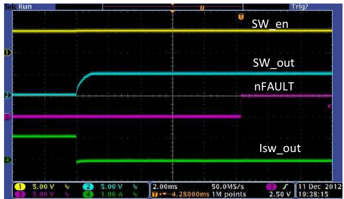
Figure 40. USB Switch Current Limit Recovery
