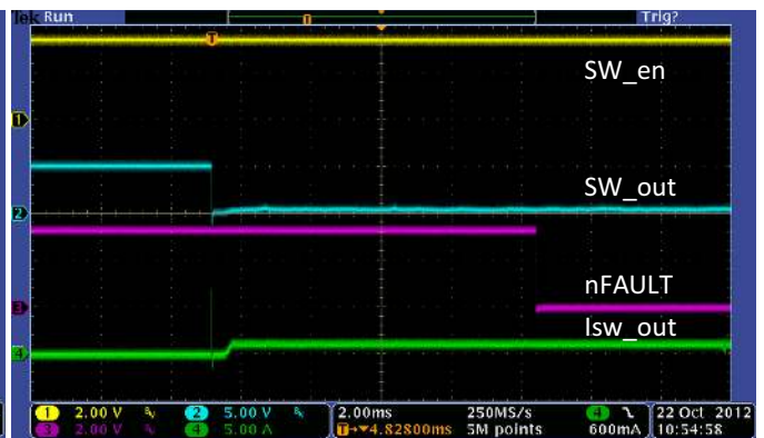
Figure 39. USB Switch Current Limit Operation
