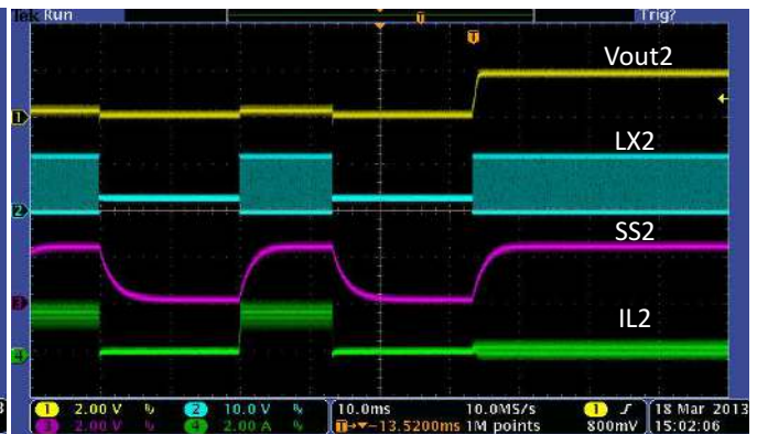
Figure 35. Hiccup Recover, Buck2=1.8V
