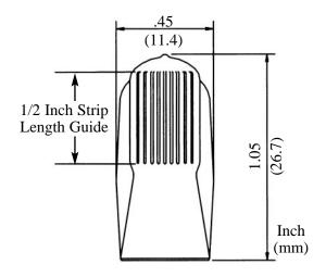
of an active (live) spring and a steel shell covered by a vinyl insulator. The spring shall have a corrosion resistant coating. (The connector shall be UL Listed and CSA Certified as a pressure cable connector. The connector shall be voltage rated 600 volts maximum, building wire, 1000 volts maximum, signs, fixtures and luminaires. The connector shall have a maximum operating temperature of 105°C.
