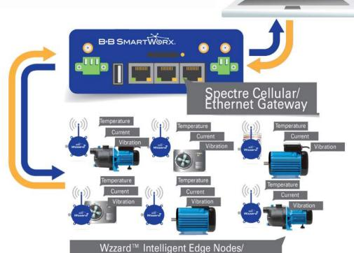
Wireless SmartMesh IP Sensor Network
