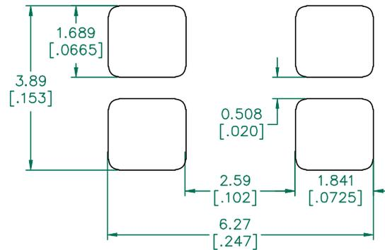
(For wave soldering, add 0.762 [0.030] to this dimension.)
