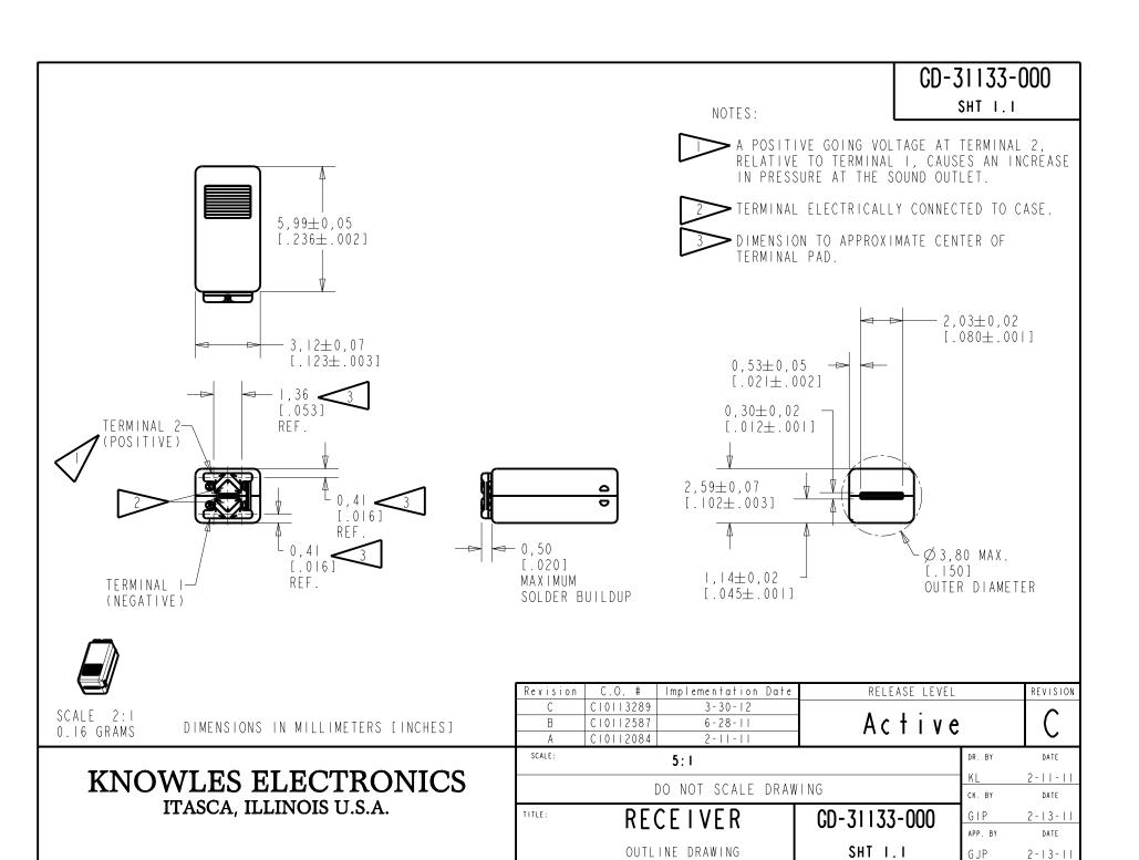
INTENDED FOR USE IN CIC, RIC, AND MINI-BTE APPLICATIONS. THIS IS A PAIR OF GE RECEIVERS WITH VERY LOW VIBRATION IN ALL DIRECTIONS. ONE GE RECEIVER IS REVERSE MAGNETIZED FOR MAGNETIC LEAKAGE CONSIDERATIONS. BOTH DAUGHTER UNITS HAVE THE CENTER TERMINAL CONNECTED TO CASE.
