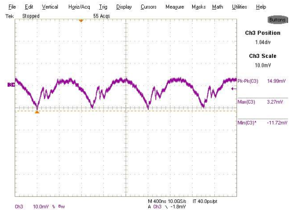
Figure 32: Output Voltage Ripple, 3A load Ch3: V out
