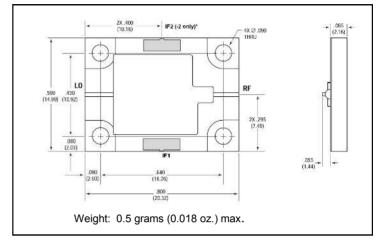
\*For the base model, only the IF1 port is connected. For the "-2" model only the IF2 port is connected.
