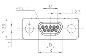
USE ABOVE FRONT FACE DIMENSIONS FOR PCB LAYOUT DESIGN. Ø0.8mm HOLE SIZE IS RECOMMENDED.
