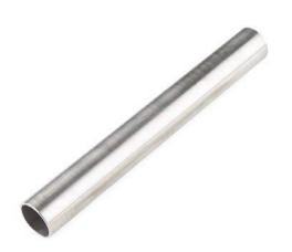
**Description:** These 8" long stainless steel tubes have an outer diameter of 1", an inner diameter of 0.88", and a wall thickness of 0.06". When used with the mating tube clamps, these can be used for versatile structural support. Additionally, wires and cables can easily be run through the center.
