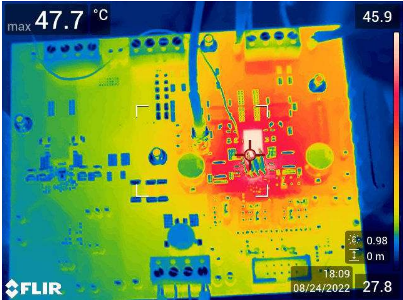
Figure 8-24. Thermal Image at 25°C Ambient
