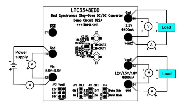
Figure 1. Proper Measurement Equipment Setup
