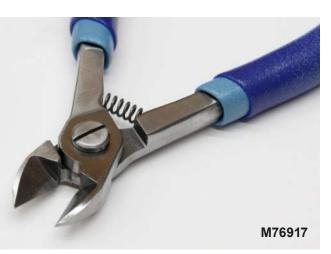
Large Oval Full Flush Cutter Designed for flush lateral cutting of heavy duty materials such as stainless steel and Nitinol up to .035".
