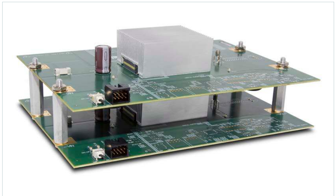
Figure 9 BCM Evaluation Boards Stacked to Form a High-Power Parallel Array, Using Common -IN and the Paralleling Connectors. Paralleling of BCM Evaluation Board.
