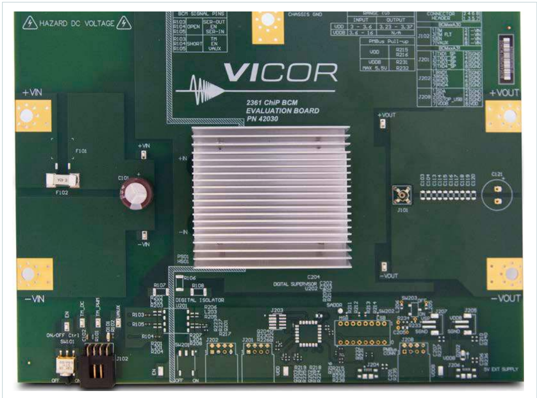
Figure 2 PCB#42030 Evaluation Board Photo, Top Side
