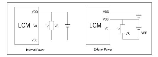
$V_{\text{DD-}}V_0$ : LCD Driving voltage VR: 10k~20k
