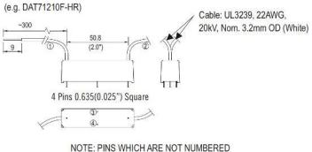
NOTE: PINS WHICH ARE NOT NUMBERED HAVE NO ELECTRICAL CONNECTION.
