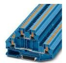
Double-level terminal block, nom. voltage: 1000 V, nominal current: 28 A, connection method: Push-in connection, 1st and 2nd level, Rated cross section:  $4 \text{ mm}^2$ , cross section:  $0.2 \text{ mm}^2$  -  $6 \text{ mm}^2$ , mounting type: NS 35/7,5, NS 35/15, color: blue
