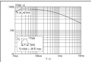
Fig.2. Maximum permissible non-repetitive peak on-state current  $I_{TSM}$ , versus pulse width  $t_p$ , for sinusoidal currents,  $t_n \le 10$ ms.
