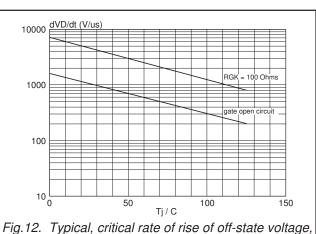
Fig.12. Typical, critical rate of rise of off-state voltage, dV<sub>D</sub>/dt versus junction temperature T<sub>j</sub>.
