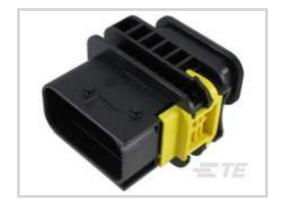
Connector & Housing Type: Housing for Male Terminals Mating Tab Width: 1.6 mm, 2.8 mm [.063 in, .11 in] Connector System: Wire-to-Wire Number of Positions: 10 Centerline (Pitch): 4 mm, 6 mm [.157 in, .236 in]
