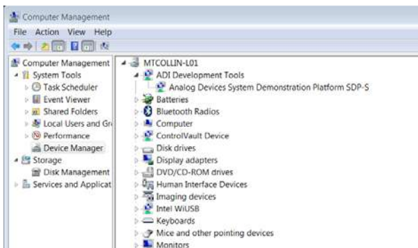
Figure 13. Device Manager: Checking that the Board Is Connected to the PC Correctly
