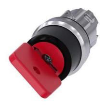
Key-operated switch O.M.R, 22 mm, round, metal, shiny, lock number 73037, red, with 2 keys, 2 switch positions O<I, momentary contact type, Actuating angle 45°, 10:30h/12h, key removal O, with laser labeling, lower case
