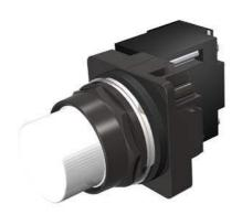
30mm BlackMax, Epoxy Coated Corrosion Resistant Complete Metal Unit Illuminated Indicator Light Transformer type, 480V AC LED Lamp, BA9s Plastic Lens, White UL Listed, CSA Certified NEMA 1,3,3R,4,4X,12,13 & Automotive Standards
