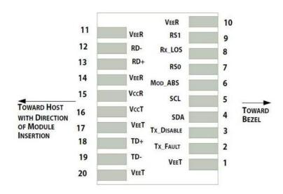
Pin-out of connector Block on Host board
