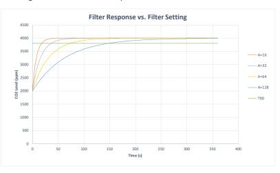
The graph above shows the effect of the filter on response times. Increasing the filter setting increases the measurement output response time.  $T_{90}$  is the time to 90% of reading. The ExplorIR<sup>®</sup>-W takes 2 readings per second.
