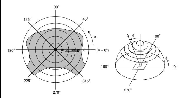
\*Are shows typ. CR≥2 (Measuring Spot:3mm)
