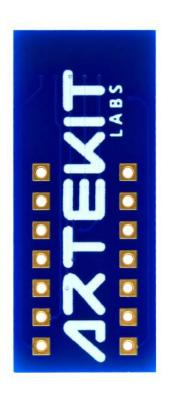
This adapter board breaks out a SOIC-14 IC with 1.27mm pin pitch into 0.1" (2.54mm) spaced pins that match most breadboards and protoboards in the market.
