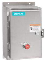
Non-reversing motor starter, Size 1 3/4, Three phase full voltage, Solid-state overload relay, OLR amp range 10-40A, 24VAC 50-60Hz coil, Non-combination type, Encl. type 4X 304 S. Steel, Water/dust tight noncorrosive, Standard width enclosure
