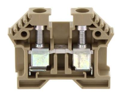
Feed-through terminal for direct mount/block variant, Screw connection, Mounting type: Mounting surface, Rated cross-section: 10 mm², Width: 8 mm, Colour: Blue
