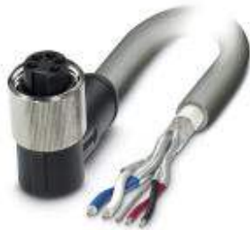
Bus system cable, DeviceNet, 5-position, PVC, Gray RAL 7001, Free cable end, on Socket angled 7/8"-16UNF, Cable length: 10 m
