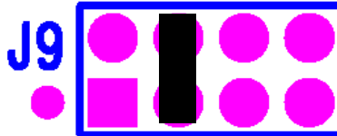
Figure 2: Output Voltage selection jumpers Jumper shown selects 1.55V output (Jumper positions from left to right are: 2.25V, 1.55V, 1.2V and 1.0V)
