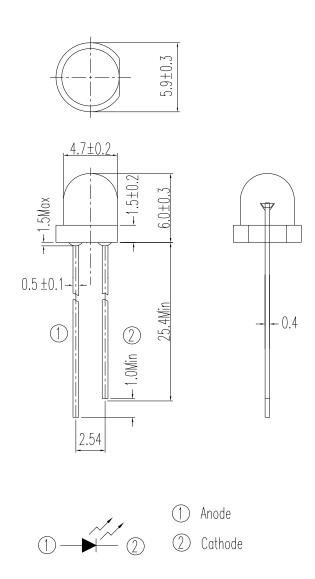
Note: Tolerances unless dimensions ±0.25mm
