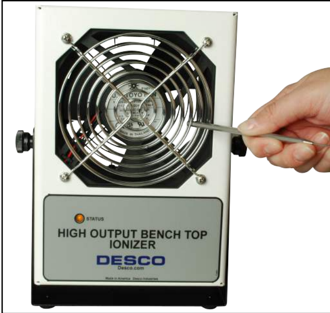
Figure 7. Shorting the ionizer's fan grill with a metal probe to test the alarm
